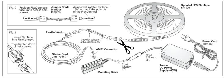
Tresco Lighting's LED FlexTape light system is designed to adhere to a smooth, clean surface (indoor locations only). To be used with Tresco DC Power Supplies Only.
