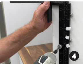
Mark your holes with tape for reference, drill first set of shelf pin holes
