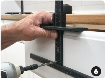
Drill hole using fixed center drill bushing (Large stop reversed for stability)
