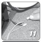
Connect the pre-stripped wires from the hose management case to the wires from the motor compartment using wire nuts (provided).
