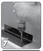
Align the bracket to the reference marks and predrill the 2 holes. Install the 2 screws through the bracket into the floor of the cabinet.
