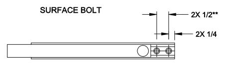
\*\*BOLTS 4" LONG (DIM "A") OR LESS ONLY HAVE ONE MOUNTING HOLE PER SIDE.
