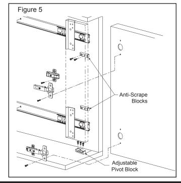
For horizontal applications, follow the mounting instructions on Page 2 for Vertical Applications/Without Partition and rotate the cabinet view 90°. See Figure 6.
