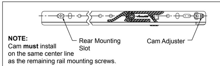
3. Connect drawer to extended slide members by lowering the drawer onto the slides so the rail rests on top of the slide members approximately 1" from the front. Pull both slides forward until the rail latch locks securely into each slide.
