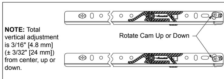
5. **IMPORTANT:** After all adjustments are made, secure rail with additional mounting screws.
