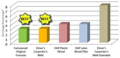
\*Volume was measured on a lab scale using the following formula: (Initial Volume - Final Volume) / Initial volume x 100 = Percent Shrinkage
