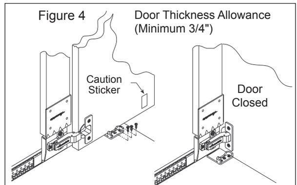
Refer to the illustrations below and the chart on page 4 to determine hinge placement for the various applications shown.
