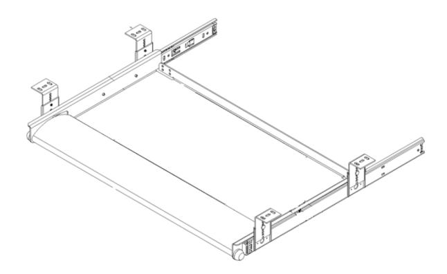
Note: Brackets mount in outboard position under work surface for application widths 24" or greater, and in the inboard position for widths less than 24"
