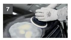
Feather around the repair area ensuring that any deep scratches are removed using a finer grade abrasive.
