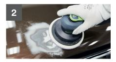
Remove paint from the damaged area using a dual action sander combined with the relevant 3M abrasive, ranging from P80 to P120 grade.
