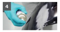
Wipe away dust and debris and apply 3M™ Polyolefin Adhesion Promoter to both sides of the repair area. Allow 10 minutes to dry.
