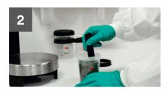
Mix colour in  $3M^{\text{\tiny TM}}$  PPS $^{\text{\tiny TM}}$  2.0 Liner, selecting the appropriate size for repair area.
