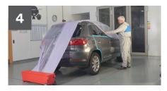
Use  $3M^{\sim}$  Masking Film to protect those large areas of the car not to be sprayed during the repair.
