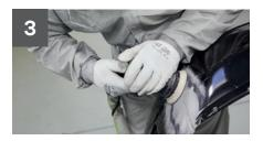
Prepare the area around the tear with a 3M™ Hookit™ Abrasive Disc P180. Avoid overheating and melting the plastic.
