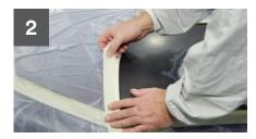
Apply the appropriate 3M masking products to suit the repair area and move vehicle into the booth.
