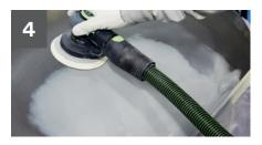
Reapply 3M<sup>™</sup> Dry Guide Coat to the panel. Machine sand using fine grade abrasives, either P400 or P500.
