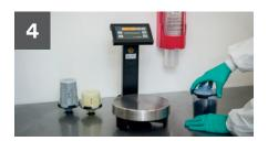
Using the 3M<sup>™</sup> PPS<sup>™</sup> Quarter-Turn Lid Locking System connect the 3M<sup>™</sup> PPS<sup>™</sup> 2.0 Lid (with built-in filter and integrated collar) onto the 3M<sup>™</sup> PPS<sup>™</sup> 2.0 Cup/Liner.
