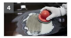
Apply 3M<sup>™</sup> Dry Guide Coat and hand or machine sand the filler to the desired shape.
