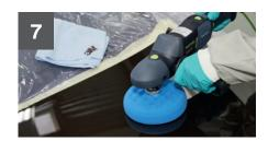
Remove holograms and swirl marks by using 3M™ Perfect-it™ Ultrafina SE Polish on a Blue High Gloss Pad. Wipe off excess compound using a blue ultra soft cloth.
