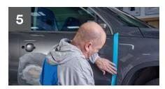
Use 3M<sup>™</sup> Scotch® Performance Masking Tape for critical areas and for general masking.
