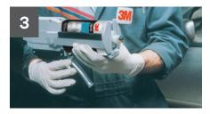
Place duo pack cartridge with adhesive in applicator. Unscrew adhesive cap and dispense enough to equalise the adhesive. Attach and lock the mixing nozzle to the duo pack cartridge.
