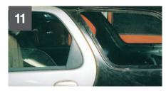
Clamps can be removed after 4 hours at 23°C and/or if there is any tension, part needs to remain clamped longer. Curing time may be accelerated by applying heat with applicator or IR lamps (do not exceed 120°C for 45 minutes). Allow 24 hours curing before returning the vehicle to service.
