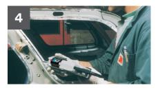
Apply adhesive bead on all areas to be bonded (all bare metal surfaces).
