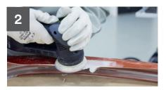
Prepare area with a 3M™ Roloc™ Disc P80 reducing the thickness of the plastic.
