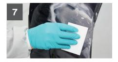
Spread and smooth 3M™ Flexible Parts Repair Material into the tear and allow to dry for 20 minutes.
