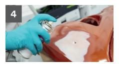
Spray 3M™ Polyolefin Adhesion Promoter on the front side of the bumper around the damaged area. Allow 10 minutes to dry.
