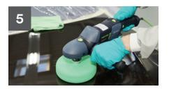
Compound the panel using 3M™ Perfect-it™ Fast Cut Plus Extreme and Green Compounding Pad. Wipe off the excess compound using a green high performance cloth.
