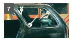
Spray 3M™ Weld Thru II Coating (50410) to all areas to be welded. Clamp the panel in its proper position.
