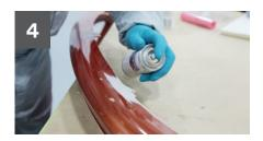
Clean the area with 3M<sup>™</sup> VHB<sup>™</sup> Surface Cleaner Cleaner and apply 3M<sup>™</sup> Polyolefin Adhesion Promoter to bare plastic area and leave to dry for 10 minutes.
