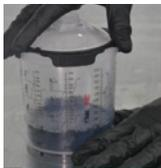
**3** Place lid on top of cup, align black portion of quarter-turn lid locking system with cup access window and push down. Twist to lock.
