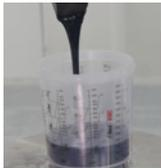
**2** Mix paint right inside the 3M™ PPS™ Series 2.0 Cup and Liner. (Note: Reduce material waste by not using a traditional mixing cup or pre-filtering.)
