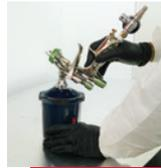
**5** When finished spraying, disconnect air line, invert gun and pull trigger to return excess paint to cup. Gently tap 3M™ PPS™ Series 2.0 Lid and Liner on a surface to help break surface tension of liquid and allow it to flow back into liner.
