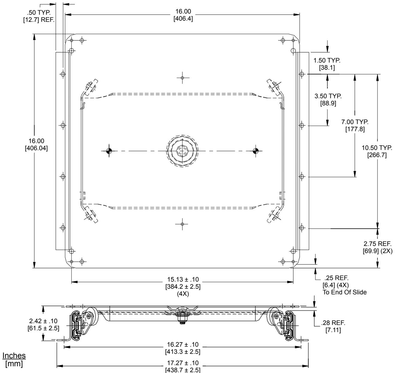
Position the swivel assembly (two slides attached to the swivel plate) on the cabinet base so the swivel platform (including the fascia) is located as far forward as possible. Swivel platform is supplied by the cabinet manufacturer or customer. The television's center of gravity should rest directly over the pivot point of the swivel or rearward. It is recommended the cabinet base and platform be a minimum of 3/4" [19.0 mm] thick.
