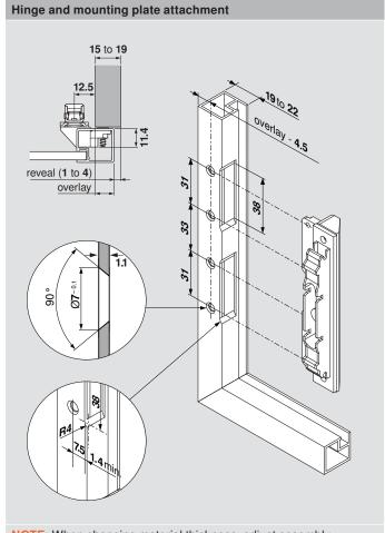
changing material thickness, adjust assembly ccordingly
