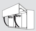
Up to three drive units can be synchronized allowing them to move simultaneously. This function is required for several cabinets with one wide front.
