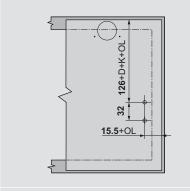
When using large overlay mounting plate (20K4501) hole location is offset by 19 (15.5 + OL - 19)
