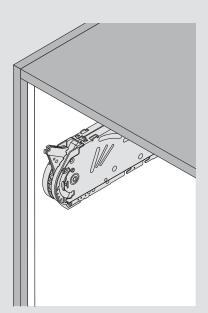
NOTE: Mounting plate position varies based on block-out thickness used at top of cabinet
