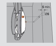
The included #7 x 35 (1-3/8") wood screws are required in the five holes marked in orange.
