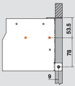
Attach bracket to face frame with two #7 x 3/4" (7074N) wood screws. Attach lift mechanism to bracket with three M4 x 30 machine screws (included).
