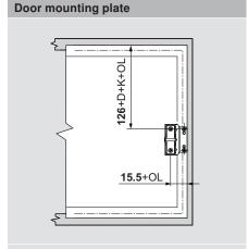
Attach using #6 x 11 (699.110) aluminum screw
