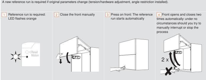
NOTE: If the reference run is interrupted, it should be reset. See reset motion on page 97 then restart reference run
