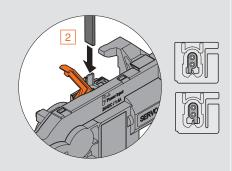
3 Once cable is inserted, press down on universal cable lock lever
