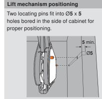
The included #7 x 35 (1-3/8") wood screws are required in the four holes marked in orange.
