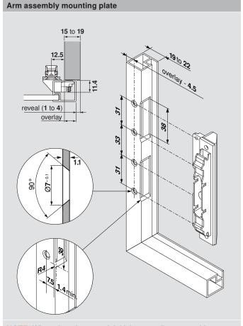
NOTE: When changing material thickness, adjust assembly dimensions accordingly
