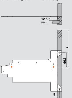
Attach bracket to face frame with two #7 x 3/4" (7074N) wood screws. Attach lift mechanism to bracket with six M4 x 30 machine screws (included).
