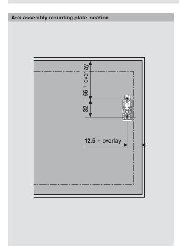
Arm assembly mounting plate choices **Mounting plate** Slab door Five-piece door more than 6 **Mounting plate with bracket** Five-piece door for large overlay five-piece doors 19 40 NOTE: Hole locations offset by 19 (example: 12.5 + overlay - 19 = hole
