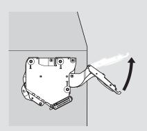
NOTE: Do not remove transport tab until just before attaching the door
