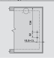
When using large overlay mounting plate (20K4501) hole location is offset by 19 (15.5 + OL - 19)
