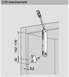
\*Location when using COMPACT 39/38C \*\*Location when using COMPACT 38N
