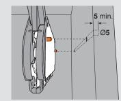
The included #7 x 35 (1-3/8") wood screws are required in the three holes marked in orange.
