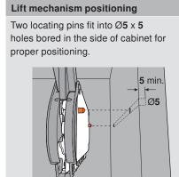
The included #7 x 35 (1-3/8") wood screws are required in the five holes marked in orange.
