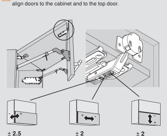
Adjust each bottom door hinge and mounting plate to properly
