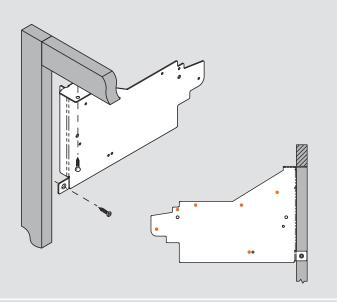
NOTE: Machine screw mounting locations marked in orange
