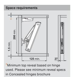
NOTE: Designed to be used in a lift up application only
