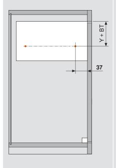
**NOTE:** Mounting plate position varies based on block-out thickness used at top of cabinet
