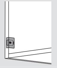
Remove battery carrier tray by pressing up or down on the battery display switch
