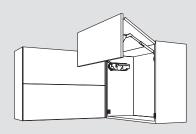
To avoid the collision of door fronts, drive units (six maximum) are linked so that only one door can be opened at a time. A door front is prevented from opening as long as a linked door front remains open.
