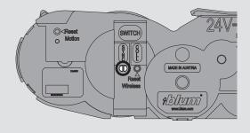
7 Collision button lights continuously.
