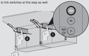
4 Confirm link by pressing flashing ok button.
