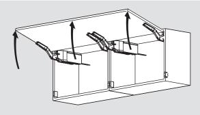
Up to three drive units can be synchronized allowing them to move simultaneously. This function is required for several cabinets with a single front.
