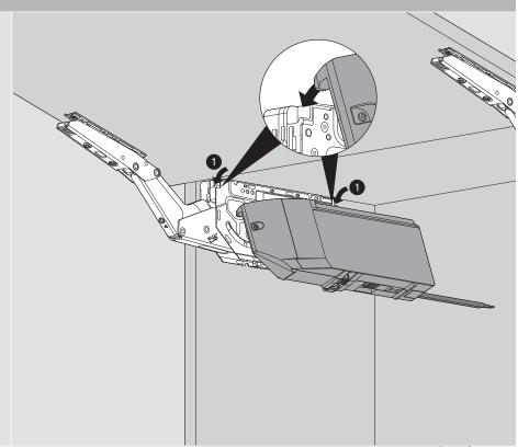
2 To lock drive unit to the lift mechanism, hold drive unit in place and press the bottom of the drive unit to click into place. Drive unit pin will self-locate during reference run.
