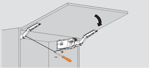
NOTE: Adjustments can be made with the cap on
