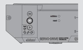
Press flashing play button to start reference run and complete synchronization.
