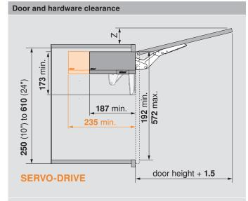
**NOTE:**  $Z = \text{door height } \times 0.29 + \text{door thickness minus}$  top frame width
