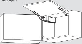
1 Press collision button on first drive unit.
