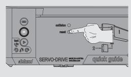
2 Link button will flash continuously when reset complete.
