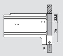
Attach bracket to face frame with two #7 x 3/4" (7074N) wood screws. Attach lift mechanism to bracket with four M4 x 30 machine screws (included).
