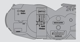
Open HK top door and press collision button on HK top drive unit.
