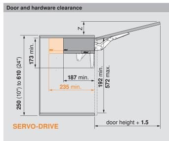
NOTE: Z = door height x 0.29 + door thickness minus top panel thickness
