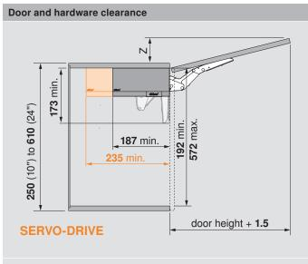
NOTE: Z = door height x 0.29 + door thickness minus top panel thickness
