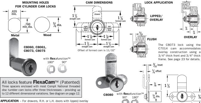
**APPLICATION** – For drawers, R.H. or L.H. doors with lipped/overlay construction (straight cam) or flush construction (formed cam). For overlay application, the combined thickness of front and frame cannot exceed the cylinder length. Also see overlay detail at above right.
