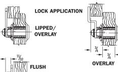
The C8053 lock using the C7014 cam accommodates overlay construction using a 3/4" thick front and 3/4" thick frame. See page 23 for details.
