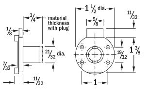
APPLICATION - Two drawer "Mini Gang" lock for desk or pedestals, and single locking drawer for desk or pedestals. Surface Mounted.
