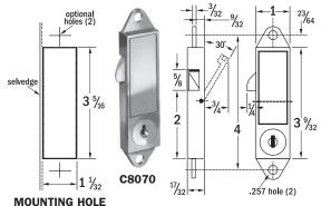
**APPLICATION** – For right handed metal doors of electrical circuit breaker cabinets.
