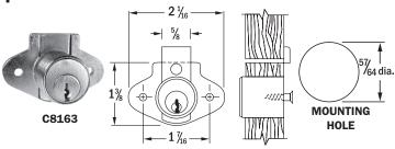
**APPLICATION** – For drawers. Surface mounted. Requires 57/64" diameter hole for cylinder.
