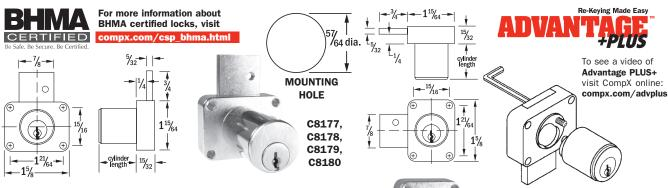
APPLICATION - For drawers, R.H. or L.H. doors. Surface mounted. Requires 57/64" diameter hole for cylinder.
