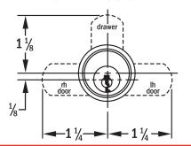
Through the use of a shifter, the 360° key turn turns the cam 90° in either direction. Actual application determines which cam position is the locked position. Each lock is furnished with an alternate cam for opposite cam turn.
