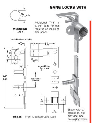
**APPLICATION** – For locking drawers in desk pedestals and other multiple drawer applications. Lock mounts in right corner. Can also be mounted for left corner application. Surface mounted. Requires 21/32" diameter hole for cylinder, and when required, a dado for bar, measuring 7/8" x 3/16" deep in inside of panel.
