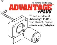
The Advantage Pus feature allows easy removal of the locking cylinder from the lock body without having to remove the lock body from the application. Simply insert a 5/64" Allen tool into the back of the lock and remove the locking cylinder from the front.
