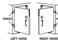
At which edge of door hinges are located determines hand of door when facing door.
