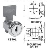
**APPLICATION** – C8701: for center drawers of metal desks. Fits special piercing of drawer front and selvedge (see drawing). C8896 is a specific replacement lock.
