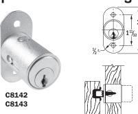
**APPLICATION** – C8140 is for sliding glass doors. C8142 and C8143 are for wood sliding doors and require a 7/8" diameter hole in front door for cylinder. C8150 is used internally on filing cabinets to gang lock drawers.
