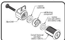
True convenience — release the key, and the self-locking component automatically returns the lock, along with SlamCAM (patent 9,605,455), to the locked position.
