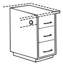
Side mounted gang lock – vertical bar movement locks all drawers simultaneously.
