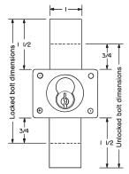
Shown in vertical function. Reverse dimensions for inverted function.
