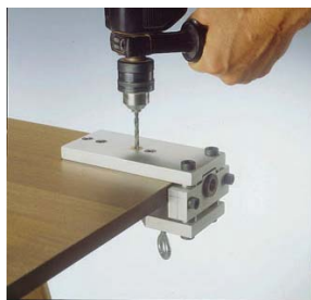
Drill the adjustment hole.
