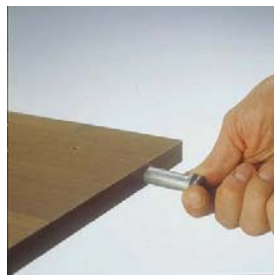
Insert 12mm Concealed Leveler into placement hole.
