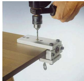
Drill the adjustment hole.
