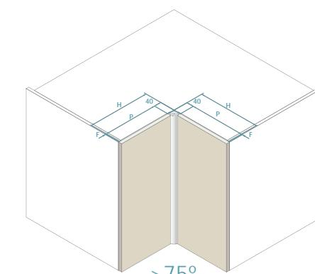
Rincoplus takes up 40 mm in 90° corners, independently of the thickness of doors. It functions perfectly for corners >75°
