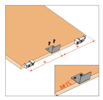
2) Fixing the magnet to the bottom.
