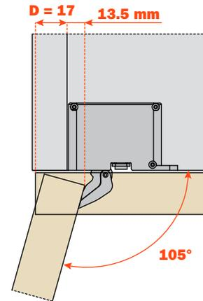
**Drilling scheme for the hinge**
