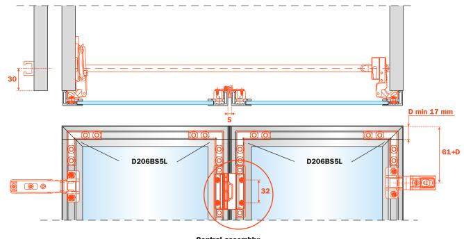
**Central assembly:** - narrow part to be mounted on the door which is fixed to the cabinet side; - wider part to be mounted on the moving door.
