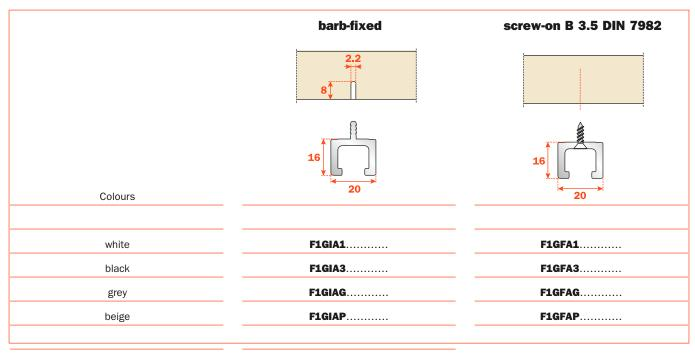
Standard lengths available: 590 mm, 880 mm, 1180 mm. Non-standard lengths can be supplied subject to a minimum order quantity of 900 pieces. The required length should be expressed in millimetres in the last four digits of the product code occupied by the dashes.
