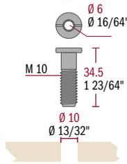
DRILLED SCREW M10 FOR SOCKET
