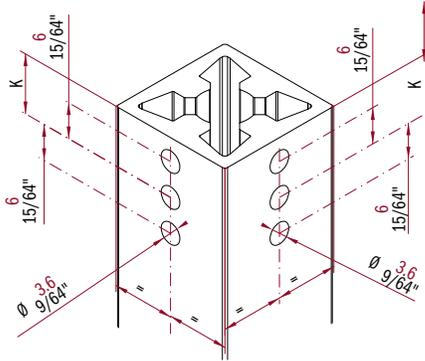
DRILLING PATTERN FOR JUNCTION BLOCK
