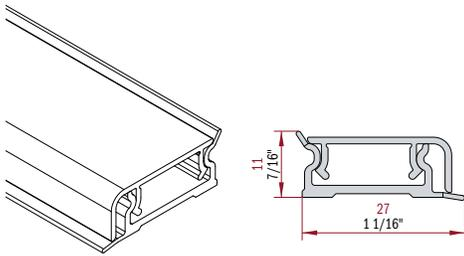
RECTANGULAR BACKSPLASH MOLDINGS PROFILE COMPOSED BY A PLASTIC CO-EXTRUDED SUPPORT PROFILE AND AN AESTHETIC PLAIN ALUMINIUM PROFILE.
