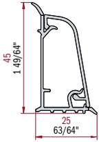
CURVED BACKSPLASH MOLDINGS PROFILE COMPOSED BY A PLASTIC CO-EXTRUDED SUPPORT PROFILE AND AN AESTHETIC PLAIN ALUMINIUM PROFILE.
