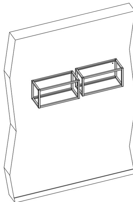
Drill a hole in the wall using a 6 mm diameter drill bit to a minimum of D. 40 mm. Insert the dowel into the hole. Fix the hook to the dowel
