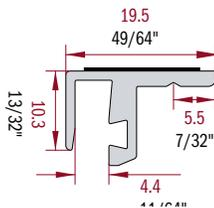
UPPER PROFILE IN ALUMINIUM FOR THE CREATION OF LATERAL AND REAR CLOSURES FOR THE SHELVING STRUCTURE.
