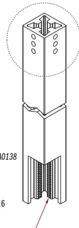
If used with leveller URCLA0138, thread M10 - 30mm - 1" 3/16 depth at the bottom edge
