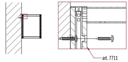
**IMPORTANT:** to cover the head of the screw or the hole diameter 8 mm, apply adhesive cover caps (not included).
