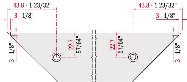
**WARNING:** It is possible to assemble the 2465 sections with the standard 45° cut using squares and screws; when adding the Plastic Corner Bumper CSP0081 an additional 3mm 90° cut is required on the edge of the sections.
