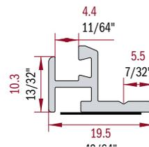
ALUMINUM LOWER PROFILE FOR CREATING LATERAL AND REAR CLOSURES FOR THE SHELVING STRUCTURE.
