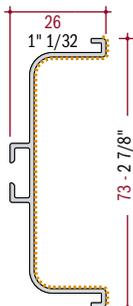
"GOLA" HORIZONTAL ALUMINIUM SPACER CHANNEL PROFILE FOR BASE CABINET
