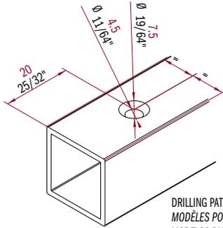
DRILLING PATTERN FOR JUNCTION BLOCK
