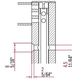
**TYPE B** - Double diameter hole. Invisible screw. Visible hole diameter 8 mm. Total adjustment 1 mm. Secure fixing to the wall.
