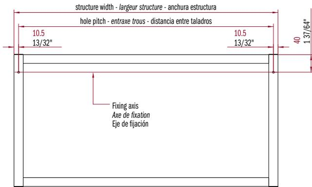
Drill through holes, diameter 4.5 mm, on the 7711 profile in the position shown on the drawing.
