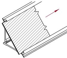
TRIANGULAR BACKSPLASH MOLDINGS PROFILE COMPOSED BY A PLASTIC CO-EXTRUDED SUPPORT PROFILE AND A PLASTIC PROFILE TO BE FINISHED WITH A STRIP OF THE SAME LAMINATE OF THE COUNTERTOP.
