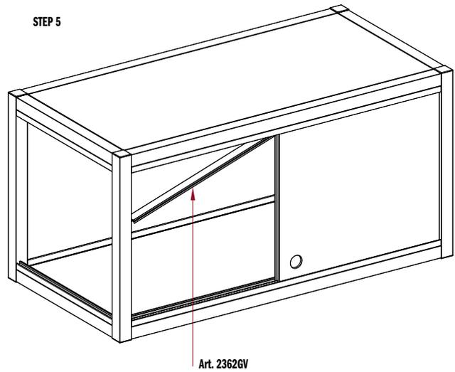
To better lock the profiles 7715; 7716; 7717 to the structure, screws can be used.
