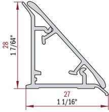
TRIANGULAR BACKSPLASH MOLDINGS PROFILE COMPOSED BY A PLASTIC CO-EXTRUDED SUPPORT PROFILE AND AN AESTHETIC PLAIN ALUMINIUM PROFILE.
