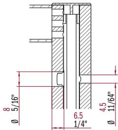
To drill the double diameter hole:
