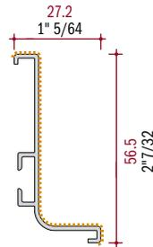
"GOLA" HORIZONTAL ALUMINUM SPACER CHANNEL PROFILE FOR BASE CABINET
