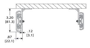
**Bottom - Mount Bracket Mounts to Top or Bottom of Cabinet**
