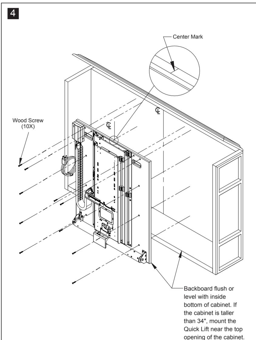
**NOTE: TOP OF THE CABINET MUST BE PARALLEL TO THE TOP OF MOVING INNER MEMBER**
