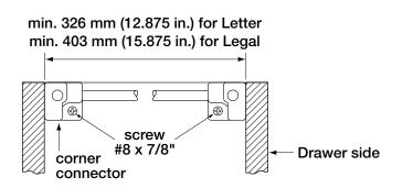
To mount FR 1811, FR 1813 or FR 1814 the location for the screw (FR 1811) or holes for the vertical rods should follow specifications as shown on drawings at right.
