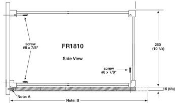
Note: A Shelf can be attached to drawer front with dowels and/or KD connector type fittings
