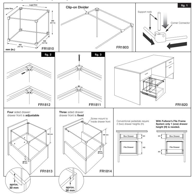
Tap support rods into corner connectors as illustrated (fig. 1). Be sure that the corner connectors face the correct direction for desired installation. You must first determine if your installation requires screw mounting to drawer front (horizontal insertion of screw (fig. 2) or to the drawer side (vertical insertion of screw, screw will break through hole fig. 3).
