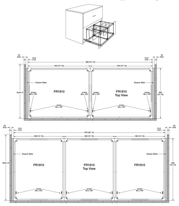
Note: C To obtain a full-extension effect with a regular extension drawer slide a minimum of 450 (18 inch) length slide is required. (FR1921, FR1020, FR2021, FR2071, FR5005 regular extension slides)
