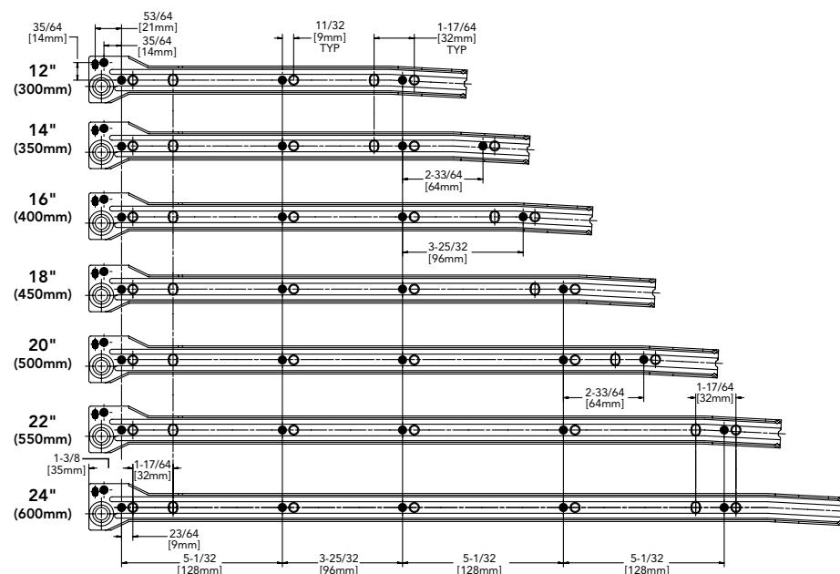
Use the #6 x 7/16" FH screws provided in the shaded mounting holes only. All non-shaded holes are intended for use with optional euro screws.
