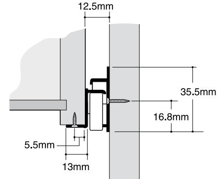
The #6 x 7/16" FH screws provided can be used in any of the shaded mounting holes.
