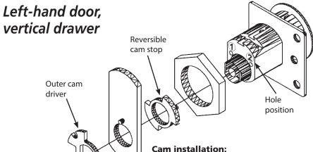
Place pin of reversible cam stop in hole #2. Place cam as pictured above. Assemble outer cam driver so that the pin from the cam is to right of the "ears." Screw in cam screw until tight.
