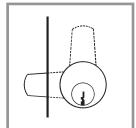
$360^{\circ}$  key rotation, key removable at cam positions 9:00 and 12:00
