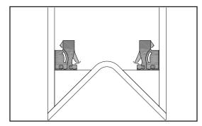
Step 4: Temporarily install the Easy Access Corner Pantry by attaching it to the inner race of the bearing with at least 2 - 1/4 - 20 X 1 flat head machine screws. Spin it and make sure it clears the inside of the cabinet and stops in the correct position. Make any necessary adjustments to the bearing location if it does not.
